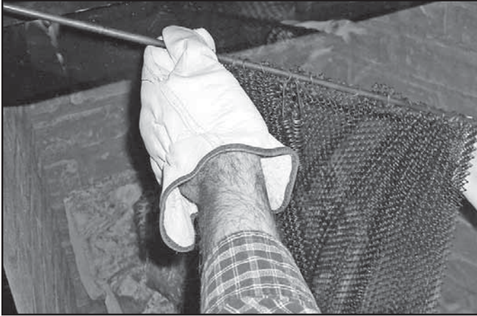
Figure 15.11 Place Left End of Screen Rod
